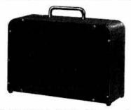
12" x 8" x 5" in 18G. Steel with Radiused Top Corners, Louvred Back and fitted with Chromium-plated 4" Handle and four P.V.C. Feet. Finished in Black, Grey or Brown Wrinkle Enamel, 18G. Steel Front Panel ... £1 Is. With Front Panel in 16G. Aluminium ... £1 2s.
