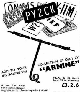
A low loss wide-band transmitting or receiving aerial. Power capacity 1 9 kW. at 7 Mc/s., '9 kW. at 14 Mc/s. Centre connection permanently sealed in Polythene moulding. Special Polythene insulators provided for suspending the Span calibrated for easy tuning.
